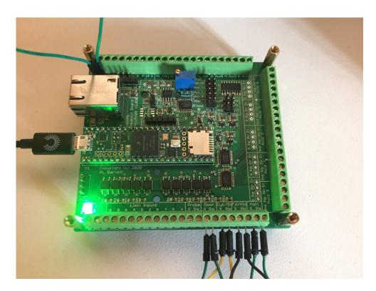
Based on a Teensy 4.1 MCU, and all manner of opto-isolated inputs and outputs included, also an ethernet interface, which I've yet to get working, but hopefully will allow a robust EMI resistant connection to the computer. It's all open source and wasn't expensive, considering how much CNC breakout boards can typically cost.
