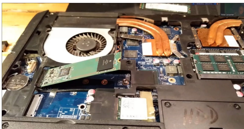
Figure 12 -Installing the 250GB M.2 SSD into the Laptop
