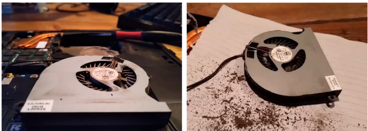
Figure 11 – The laptops fan assembly before and after cleaning.
