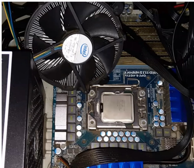
Figure 9 – A clean CPU & heatsink-fan combination ready for thermal paste and assembly
