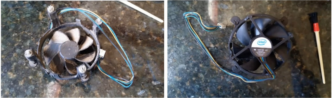
Figure 6 – Heatsink fan before and after cleaning
